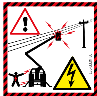
CODE: LBL-ELECT EU DANGER ELECTROCUTION HAZARD WATCH FOR OVERHEAD POWER LINES
