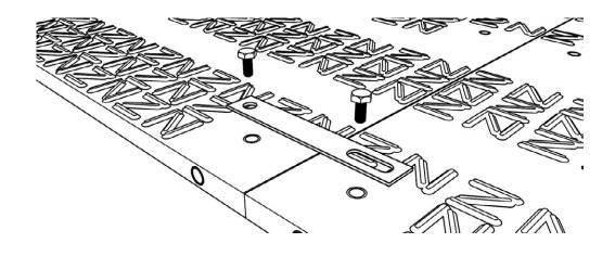
Care should be taken when laying the panels to ensure that they have the same profile side facing up.
