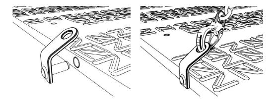
The panel is transported or laid in the desired position by tightening the chain sling so that it can then be bolted.
