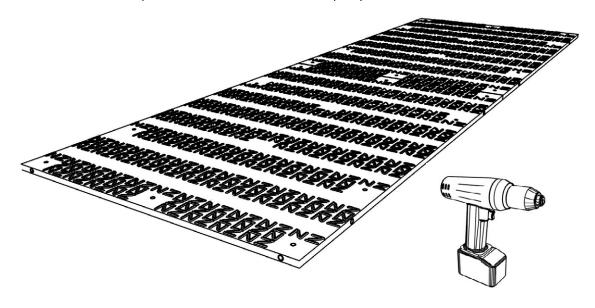
It is advisable to use a cordless screwdriver to connect the M16 screw. Alternatively, this can also be done with a hand ratchet. With both assembly options a screw attachment (24 spanner socket) should be used so that the panels can be bolted to the connection lugs provided.
