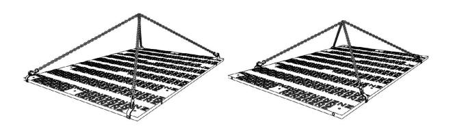
Insert the load-bearing hooks in the lifting lugs on the side to be able to move the panel optimally using a chain sling and to bring it into the desired position.
